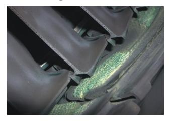
HP Seal Segments showing severe thermal erosion
