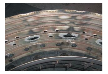
Combustor Outer Wall showing extreme overheating
