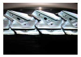
HP turbine blade showing gross erosion of shroud and front seal fin
